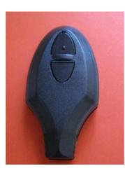
3. Once buttons pad is fitted in you will place it over part of shell with electronic board inside, press it till it closes firmly. Position screws in holes at the back and screw it together.
